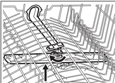
3. Wash the spray arm under running water. Use a thin pointed tool, e.g. a
